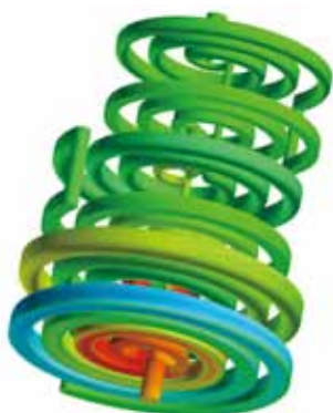
Double corkscrew mixer flow path diagram
