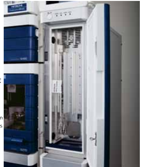
A view of column oven accommodating columns
